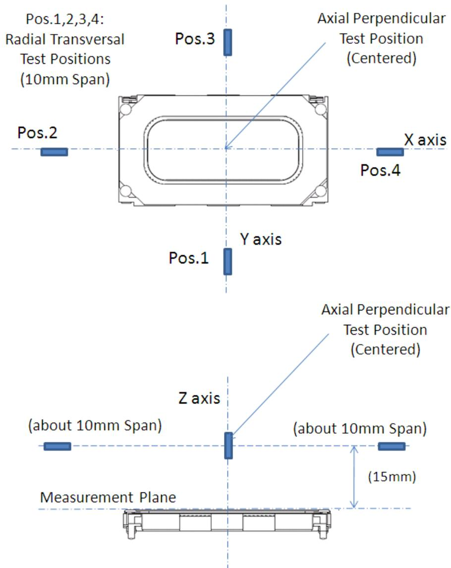
*\*Receiver must be mounted on a **plastic** surface, magnetic ambient levels be low as to not significantly affect the measurement, magnetic shielded chamber would be better.*
