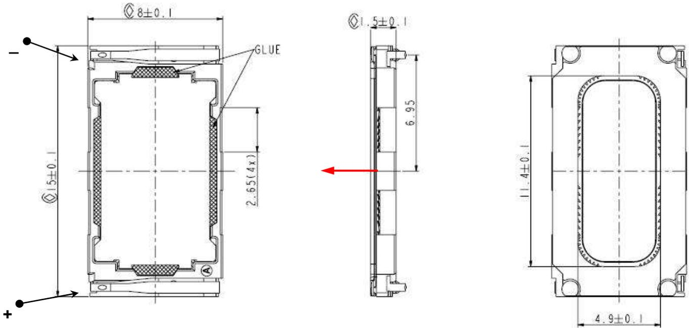
Positive voltage on pin '+' moves membrane in direction of red arrow!
